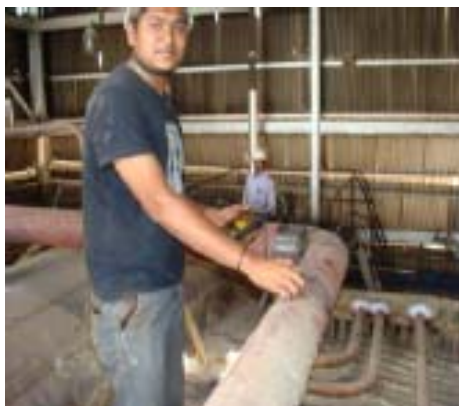
Thickness measurement in Saturated Steam line
