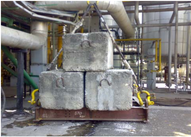
Chain block being tested
