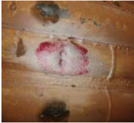
Dent mark observed in D-Panel Roof Tubes
