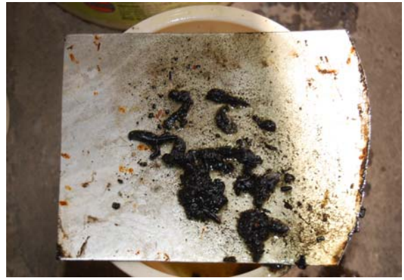
FIG 6, Black deposits removed from Console
