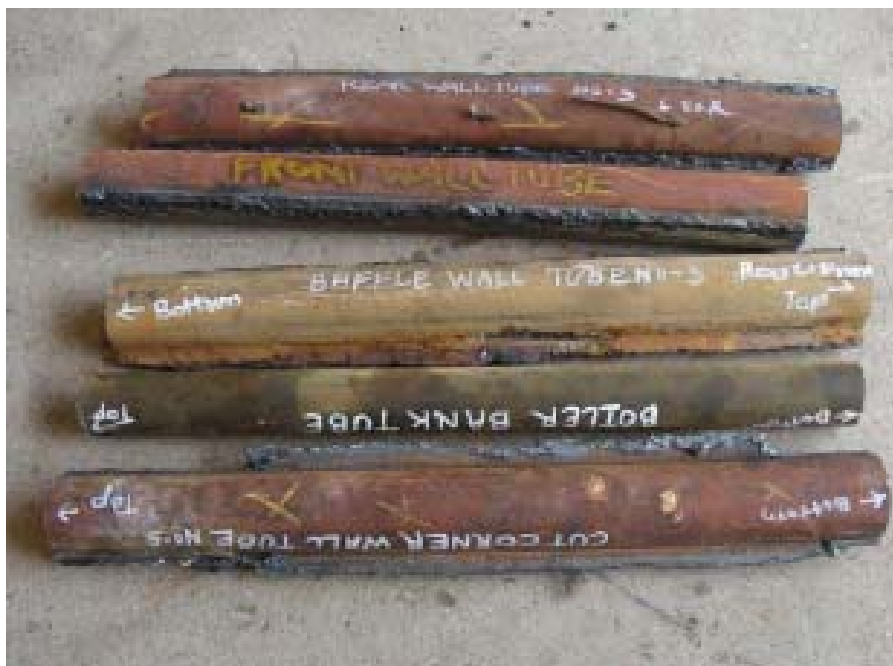
Tube samples cut from various locations for destructive testing
