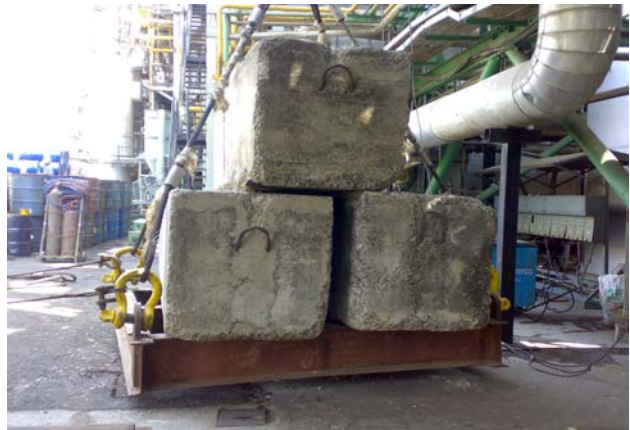
Chain block being tested
