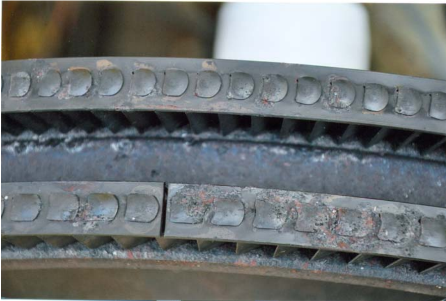
FIG 7, – View of wheel of removed rotor of turbine
