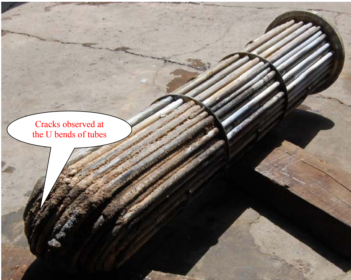
DAMAGED U-TUBE BUNDLE OF 103-JAT/JBT GLAND CONDENSER
