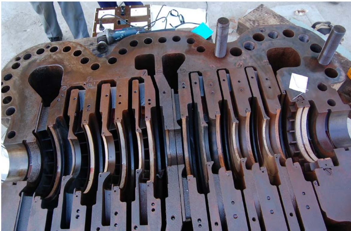
101-JHP TOP CASING CLEANING UNDER PROGRESS
