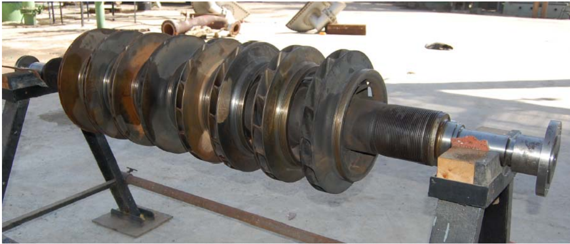
REMOVED 101-JHP ROTOR ASSEMBLY INSPECTION UNDER PROGRESS
