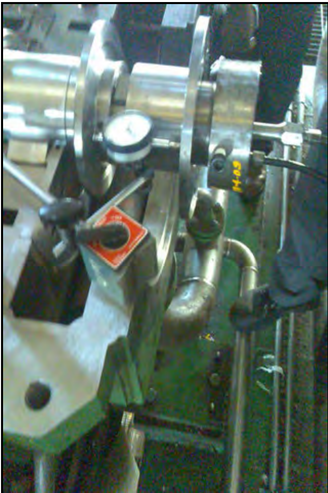
Installation of Coupling Half
