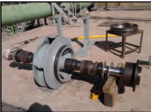
Repaired and painted Cooling water Pump Impeller
