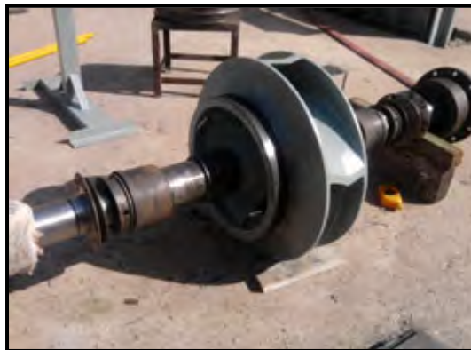
Repaired and painted Cooling water Pump Impeller
