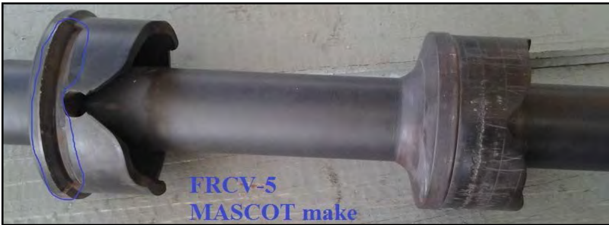
Damaged seating part of FRCV- 5
