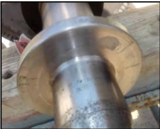
Scoring on Thrust Collar of Turbine
