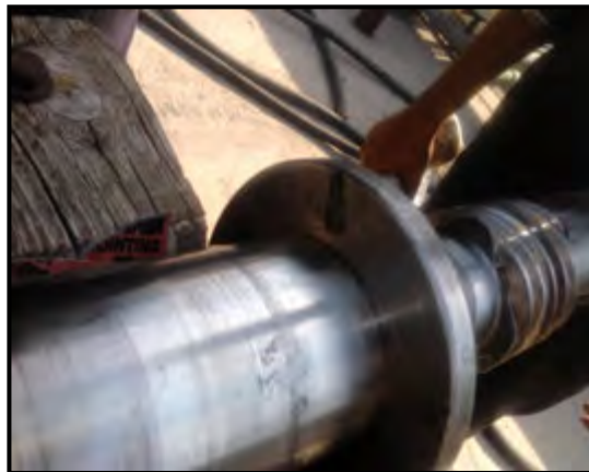
Scoring on Thrust Collar of Turbine
