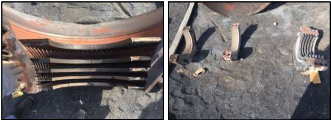
Cleaning of rotor and diaphragm assembly.
