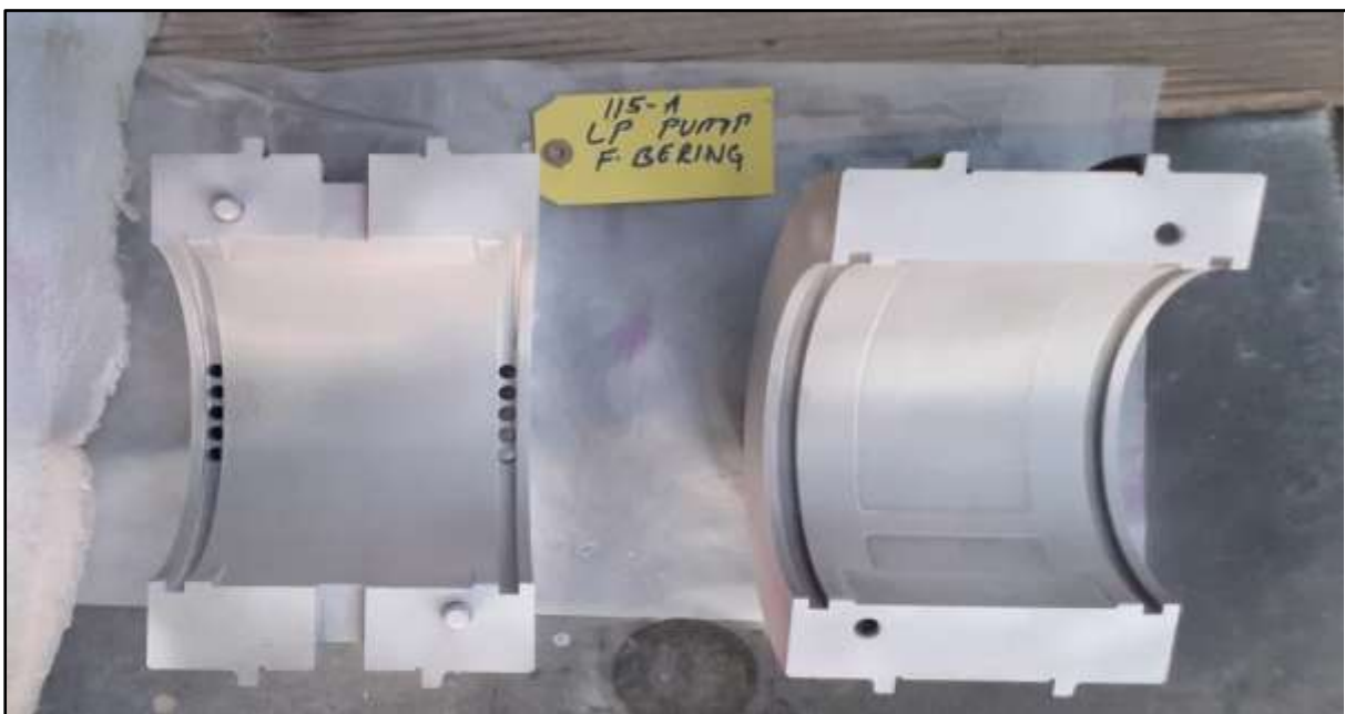
Pump Front bearings DP test conducted.
