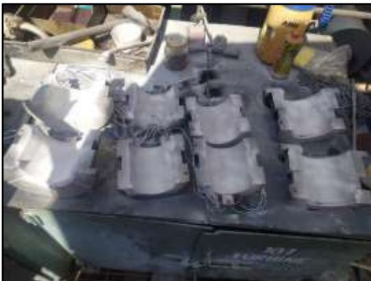
Gear wheel & pinion wheel bearing pad DP test
