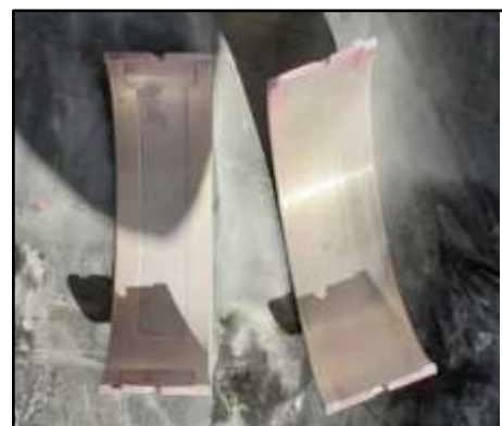
Turbine Front & Rear bearings DP test conducted
