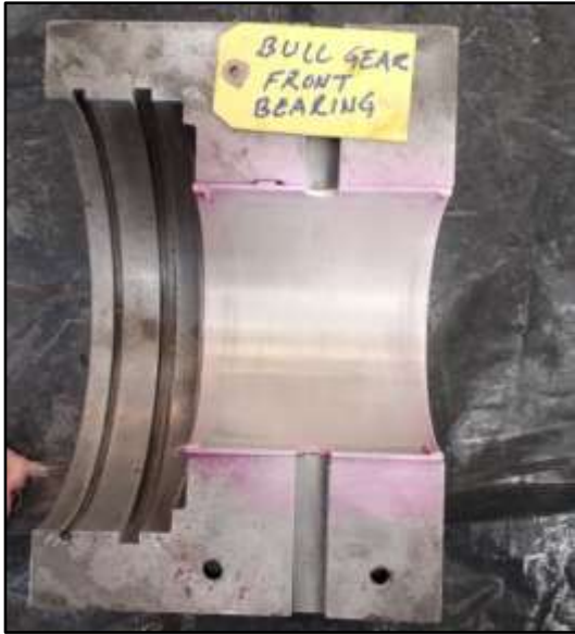
Gear wheel bearings DP test conducted
