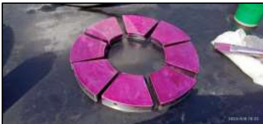
Gear wheel & pinion wheel bearing pad DP test
