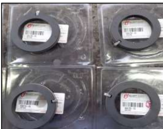
Rotor Front & Rear carbon seals replaced with new ones.
