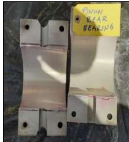
Pinion bearings DP test conducted.
