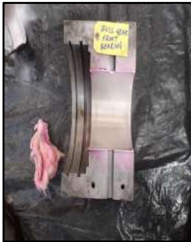
Gear wheel bearings DP test conducted
