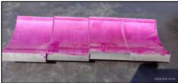
Turbine front journal bearing pads DP test conducted
