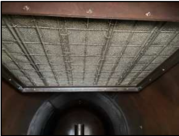
Standpipe cover plate detached from here and laying on bottom of the shell
