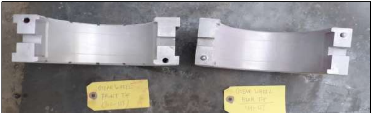
Gear wheel bearings DP test conducted
