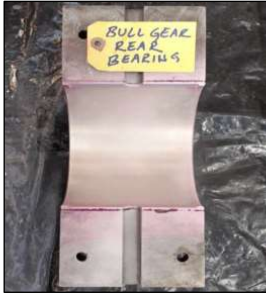
Gear wheel bearings DP test conducted
