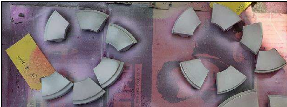
Turbine thrust pads DP test conducted
