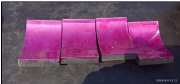
Turbine Rear Journal bearing Pads DP test conducted
