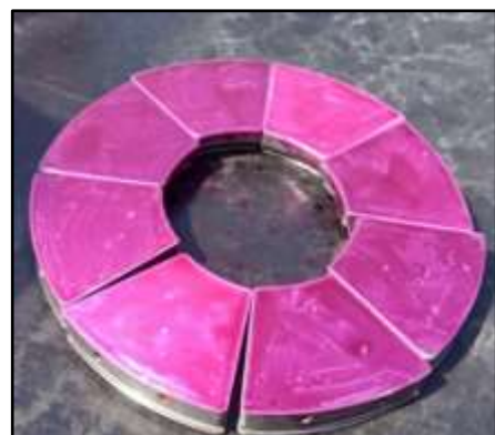
Turbine Rear Journal bearing Pads DP test conducted
