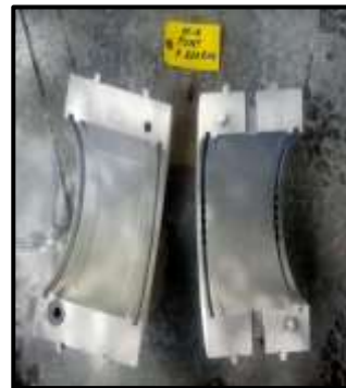
LP-Pump Front & Rear bearings DP test conducted
