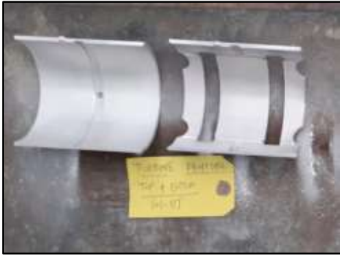
Turbine Front & Rear liner bearings DP test conducted
