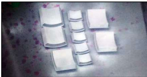
HP Compressor Front and Rear Journal Bearing pad DP test
