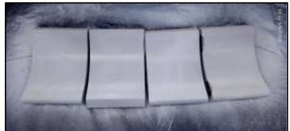
Turbine Rear Journal bearing Pads DP test conducted
