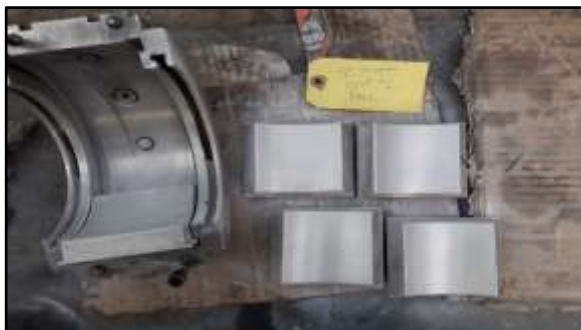
LP compressor front journal bearing pad DP test & gauss test
