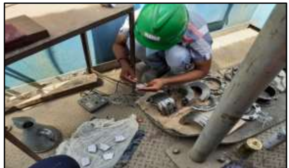
LP compressor front journal bearing pad DP test & gauss test
