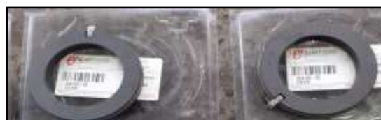
Rotor Front & Rear carbon seals replaced with new ones.
