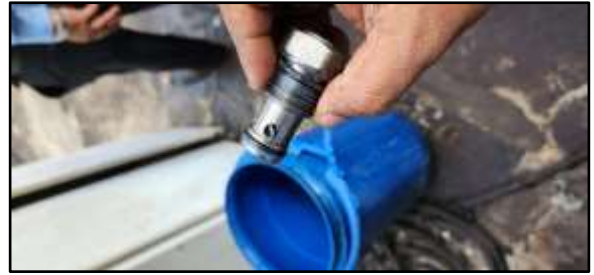
O-ring particle got stuck in NRV
