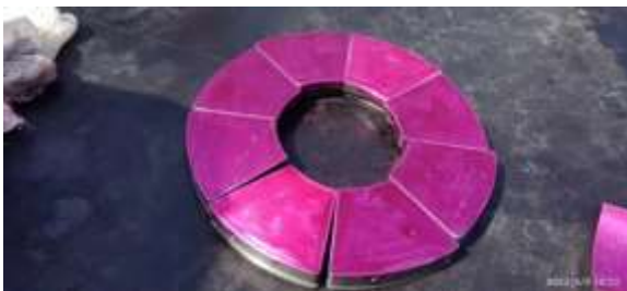
Turbine Active/Non-active thrust pads DP test conducted.
