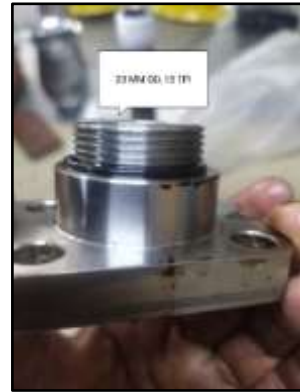
QCNRV was replaced with new spare one with modification in tapping thread
