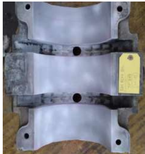
Gear wheel bearings DP test conducted
