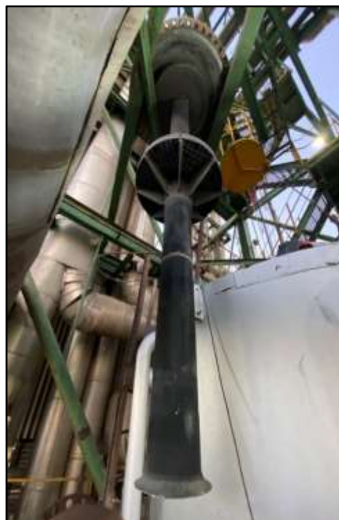
Top Cover with Air Mixer Nozzle
