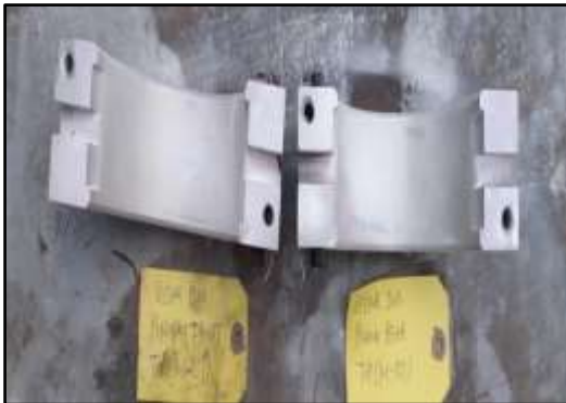
Pinion bearings DP test conducted
