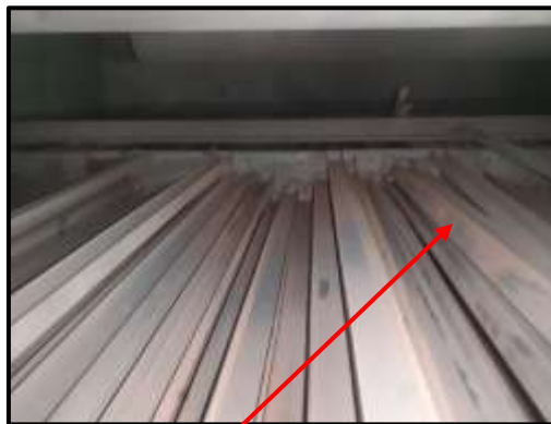
Tray Segments found dislocated from its position
