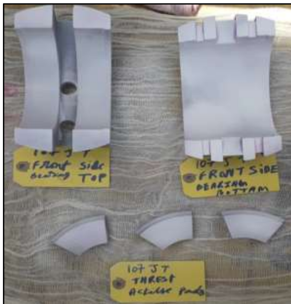
Turbine Front bearings, Active side thrust pads DP test done.
