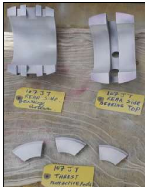
Turbine Rear bearings, Non-active side thrust pads DP test done
