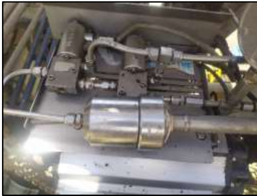
QCNRV was replaced with new spare one with modification in tapping thread
