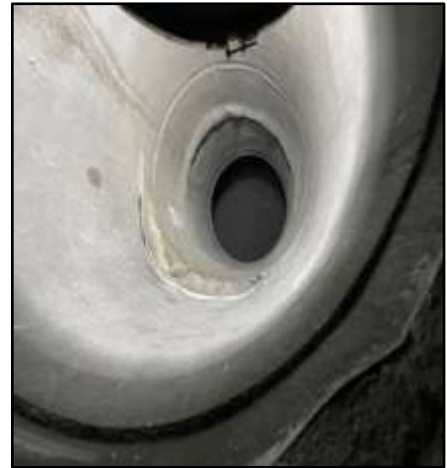
Extended portion grinded off
