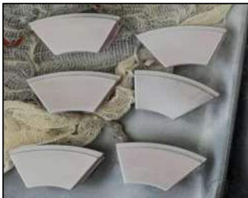
Turbine thrust pads Active/Non-active DP tests conducted
