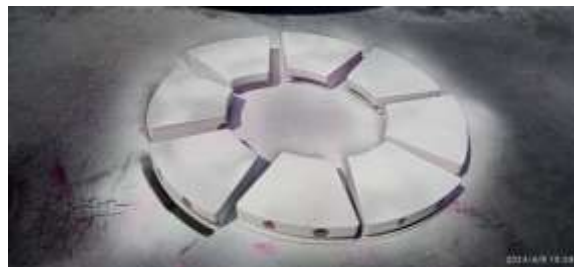
Turbine Active/Non-active thrust pads DP test conducted.
