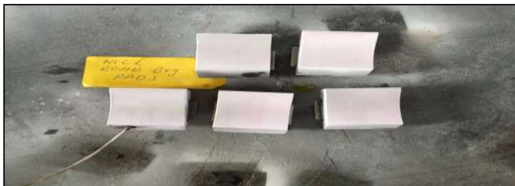
Tilting pad of Journal Bearing after DP test.
