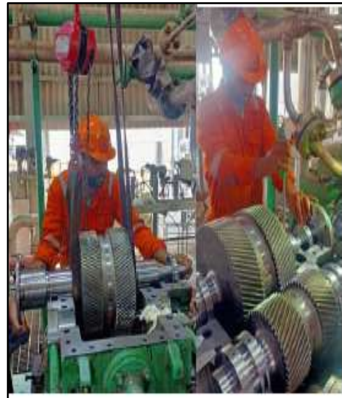
Complete Gearbox assembly before boxing up
