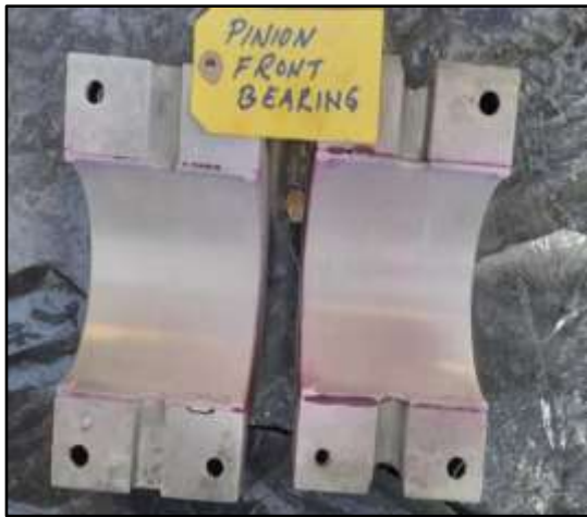
Pinion bearings DP test conducted.
