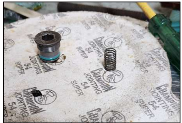
Dismantled the NRV and removed the particle and assembled.
