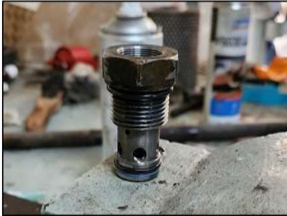
Dismantled the NRV and removed the particle and assembled.
