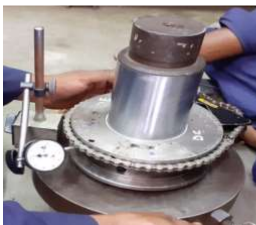
Turbine/LP/HP Compressors DE/NDE Bearings clearances checked by Mandrel Method.
