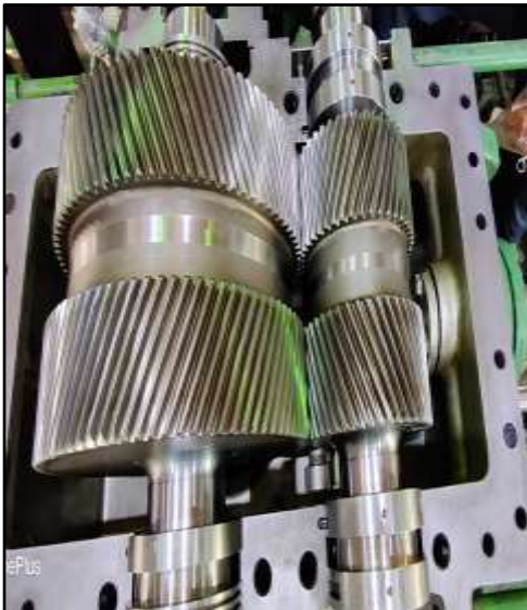
Complete Gearbox assembly before boxing up
