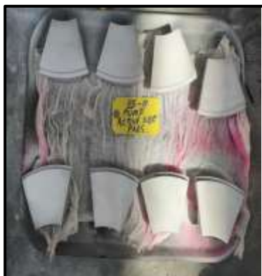
LP-Pump thrust pads Active/Non-active DP test done.
