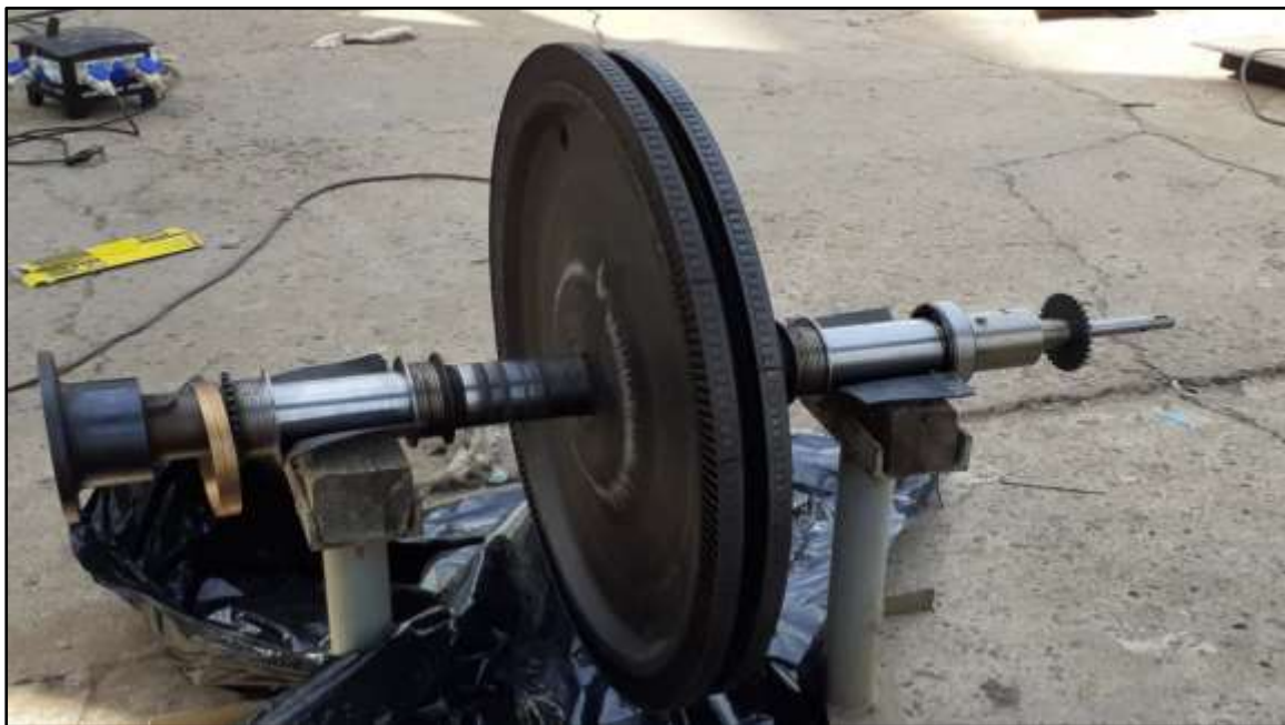
Turbine Rotor opened from its position.
