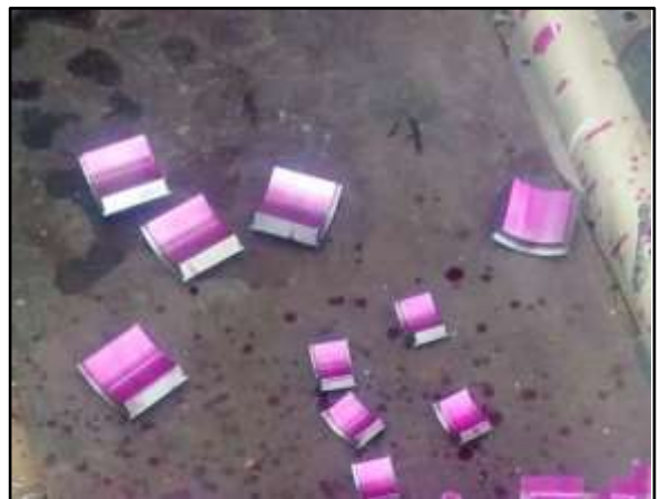
HP Compressor Front and Rear Journal Bearing pad DP test
