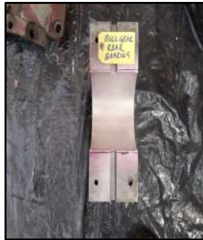
Gear wheel bearings DP test conducted
