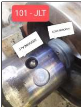
Turbine Trip pin broken
