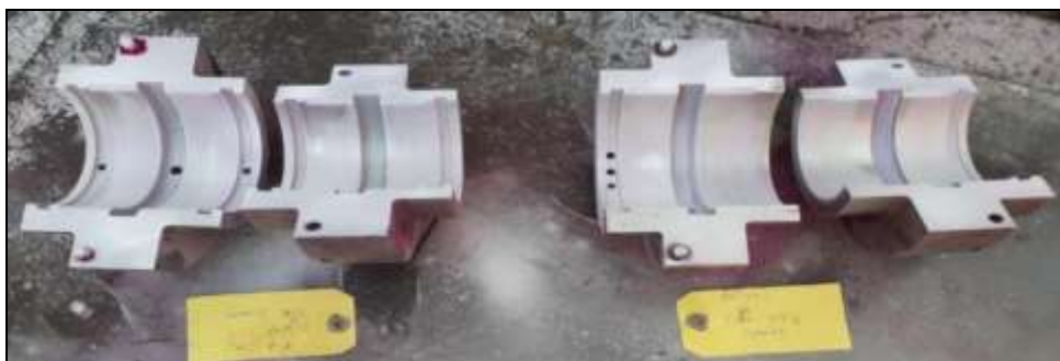
Pump DE/NDE bearings DP test conducted
