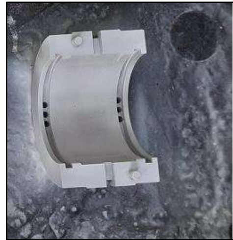
Pump Rear bearings DP test conducted
