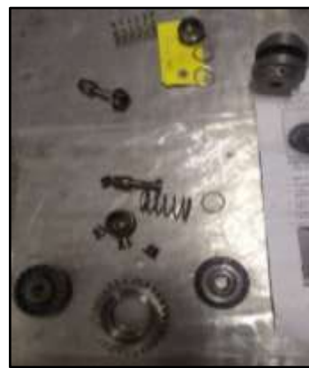
Complete trip assembly replaced
