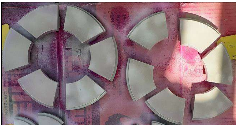
Pump thrust pads DP test conducted
