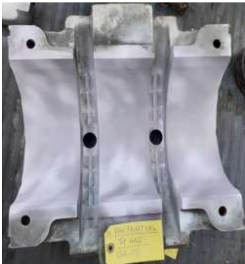
ID Fan Front & Rear bearings DP test conducted
