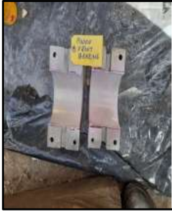
Pinion bearings DP test conducted
