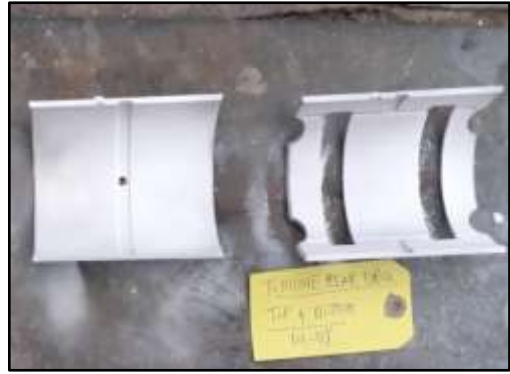
Turbine Front & Rear liner bearings DP test conducted
