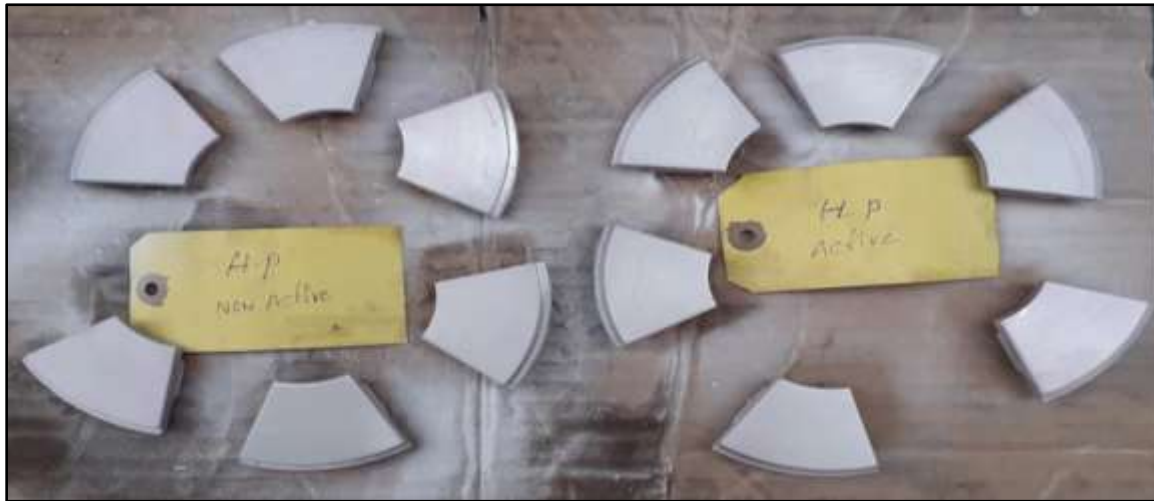
HP Compressor Rear thrust Pads (Active/Non-Active) DP test conducted
