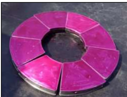
Turbine Rear Journal bearing Pads DP test conducted
