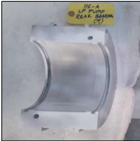
Pump Rear bearings DP test conducted
