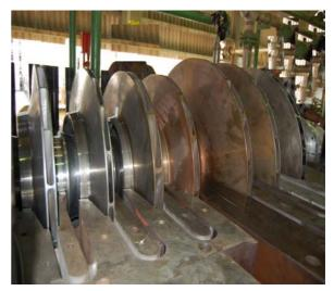
LP Compressor rotor kept on bottom casing
