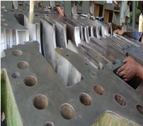
**LP Compressor bottom casing after cleaning**
