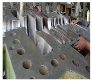
LP Compressor bottom casing after cleaning
