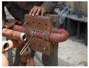
Fig. 19 Fit-up for Tacking
