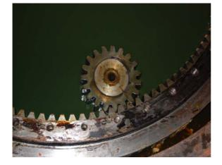
Spur gear engaged with Gear Wheel
