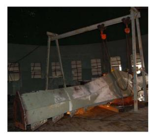
Lifting arrangement for Scraper
