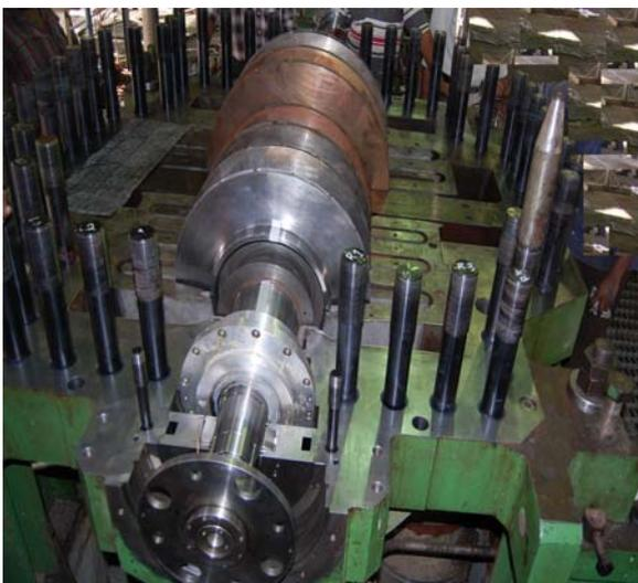
**LP Compressor rotor placed in position**
