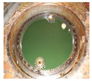
Gear Wheel and Spur gears
