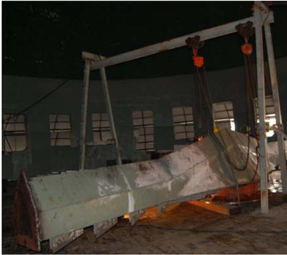
**Lifting arrangement for Scraper**
