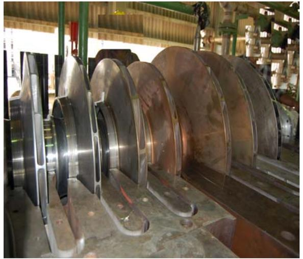
**LP Compressor rotor kept on bottom casing**
