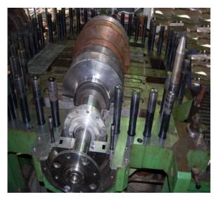
LP Compressor rotor placed in position
