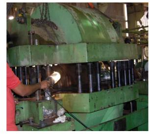
Boxing up of top casing of LP Compressor
