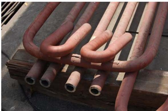
**Fig.17 Cut Pieces from PSH Coils**
