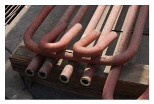
Fig.17 Cut Pieces from PSH Coils
