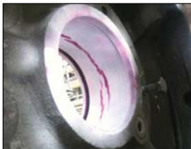
Old Cracked Stuffing Box
