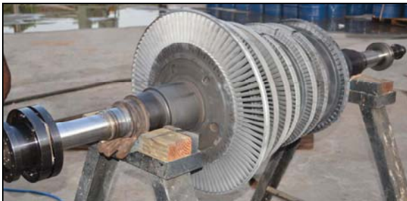
103-JBT ROTOR CLEANED BY SAND BLASTING
