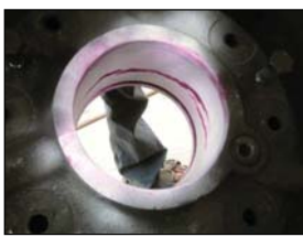
Old Cracked Stuffing Box
