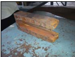
Corroded frame of level gauge glass
