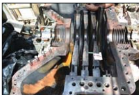
Bottom Casing & diaphragms of Elliott Turbine
