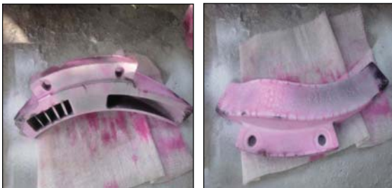
Old Cracked reversing Chambers
