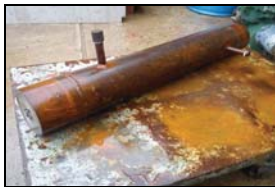
Mock-up test piece for hydro testing to check tube to tube sheet expansion joint
