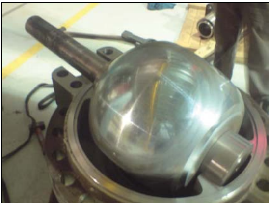
USV – 933 Control valve Plug and seat after dismantling
