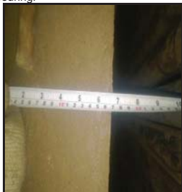
NEW REFRACTORY 165 MM THICK AS SHOWN IN SKETCH
