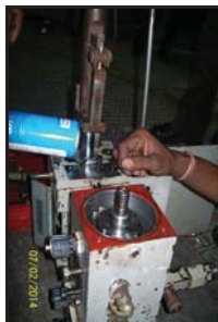
Pilot valve – after removal of top cover
