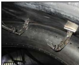
Thermocouple was bent upwards and a plate was provided for supporting the thermocouple.
