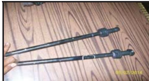
Step marks observed in spindle ( L ) - area shown by white marker
