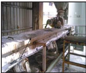
SS skirt block holding system with SS Cover
