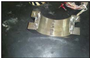
Gear box – high speed bearing (lower half)
