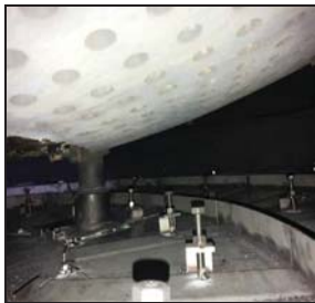
3 rd bed protection screen after installation
