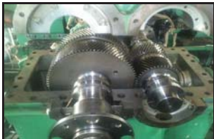
Gear box – top cover removed
