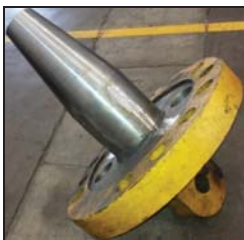
Lifting cover inside which taper plug was welded
