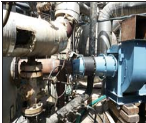
The suction of portable blower was taken from opening at skirt at convertor bottom
