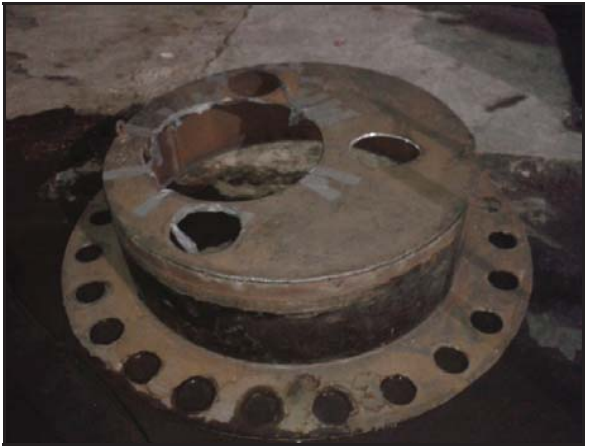
Manhole cover was pre fabricated as per drawing given below for covering top of Pressure shell
