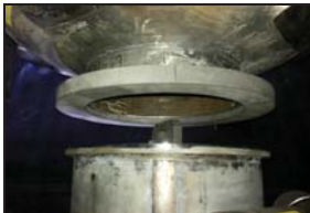
Gap between inner collector top and end of 122-C
