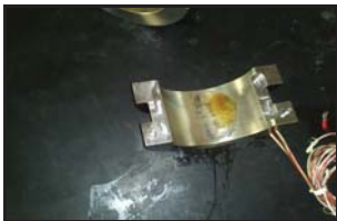
Gear box – high speed bearing (lower half)
