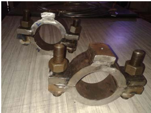
Clamp for HT Superheat Coil Skin Temp.
