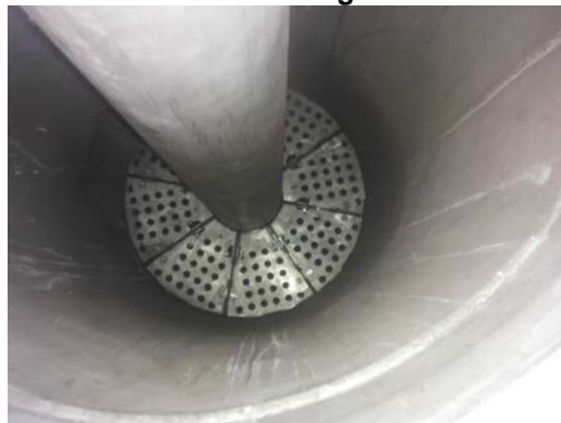
Checking restriction between distribution grids and liner
