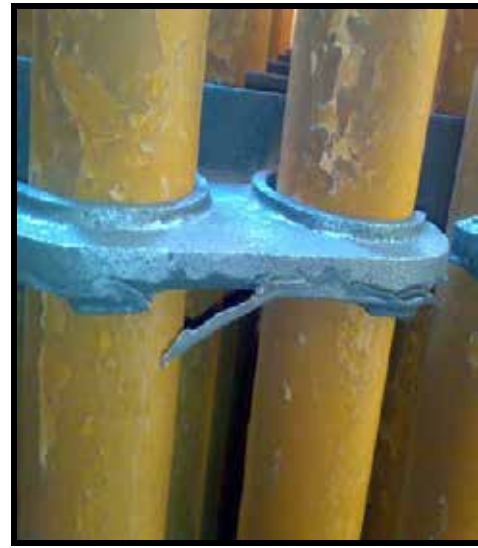
Metal peeled off in anchor supports
