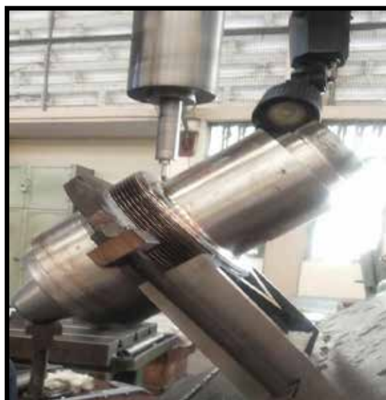
LRCV-1201 Bonnet modification for continuous flushing path
