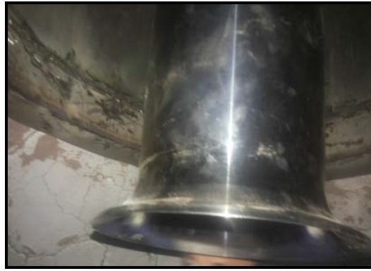
Circumferential ring in L shape welded on bottom of neck of 103-D
