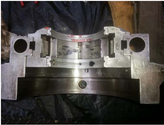
LP Compressor Thrust End Journal Brg
