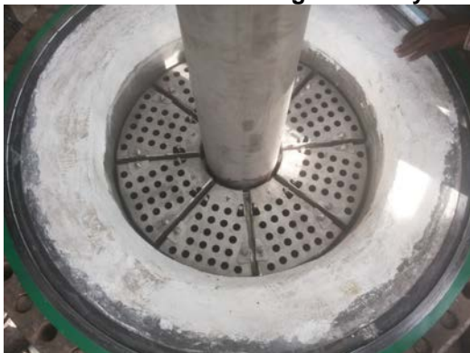
Checking restriction between distribution grids and liner
