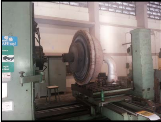
Old Burner Pipe was cut & Bevel edge made on Boring Machine
