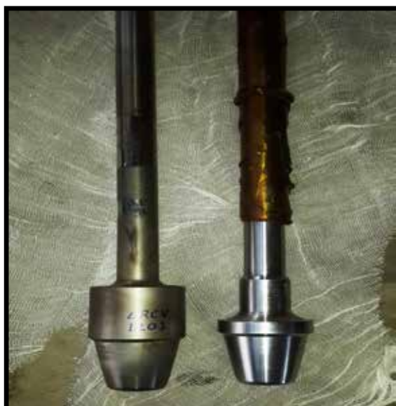
LRCV-1201 Plugs Old and New Modified to reduce side thrust
