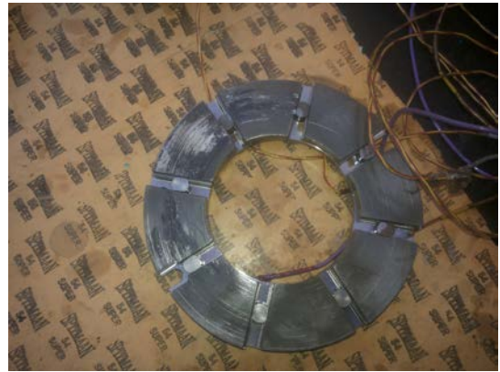
LP Compressor Thrust Bearing
