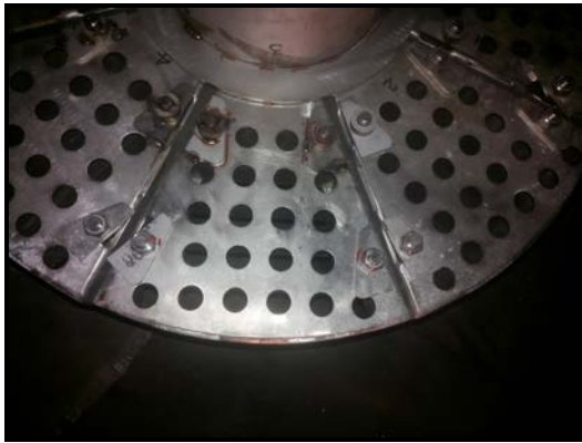
Tack Welding of Nuts to the bolts & fixing pins to the washer
