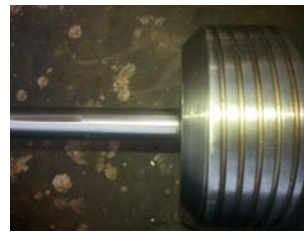
Scoring mark on Piston rod
