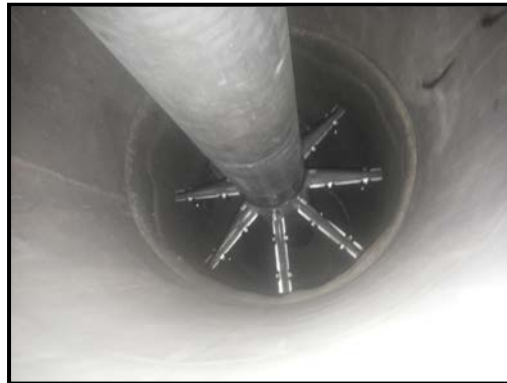
Circumferential ring in L shape welded on bottom of neck of 103-D
