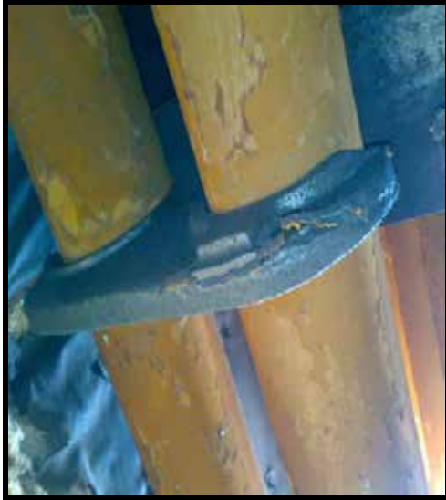
Metal peeled off in anchor supports
