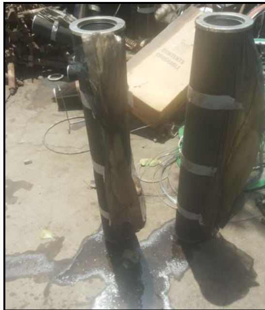
Damaged Filter cartridge of 101-J LO Console
