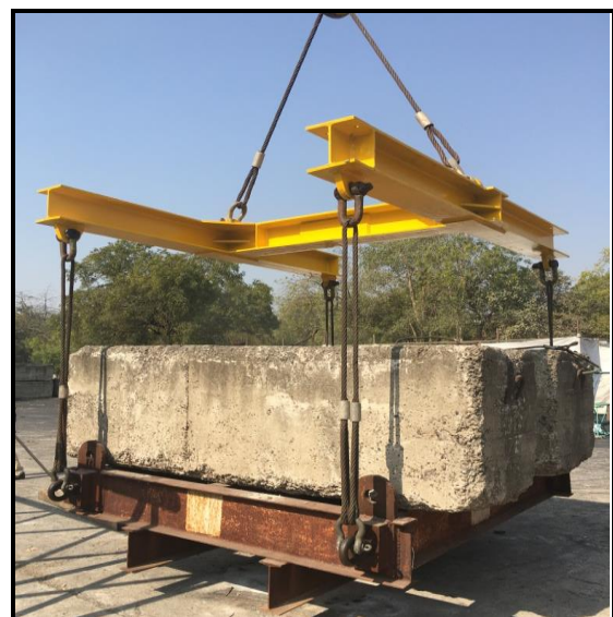
Lifting of load in eye bolt testing arrangement
