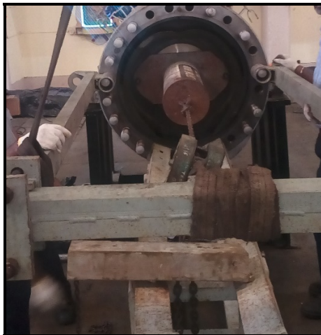
Bundle being pulled out from barrel
