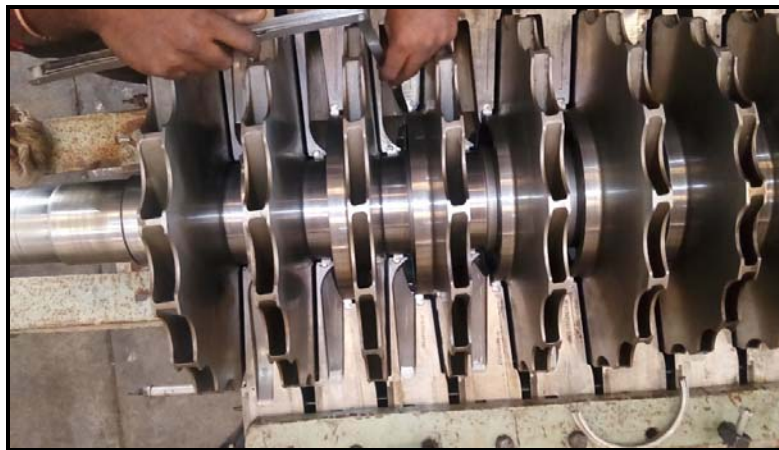
Measuring Clearance of bottom half
