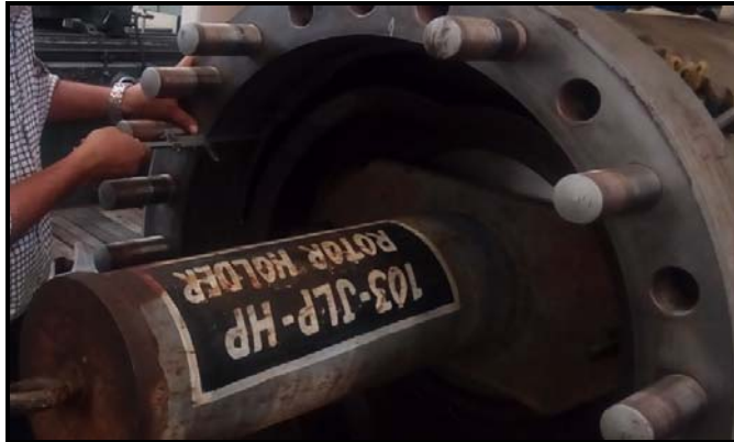
Insertion of bundle in casing
