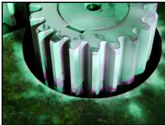
Dye penetration test of gear teeth
