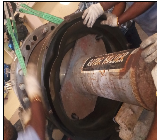
Bundle being pulled out from barrel
