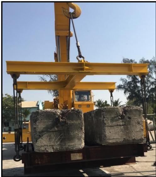
Lifting of load in eye bolt testing arrangement
