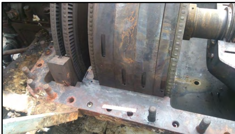
#1 Diaphragm was found rotated slightly from position
