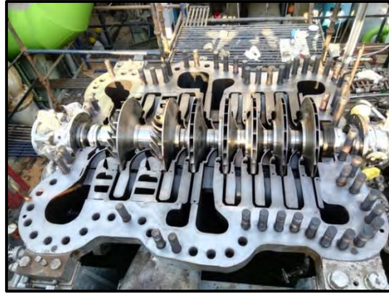
Clearance measurement & preparation for final Assy.
