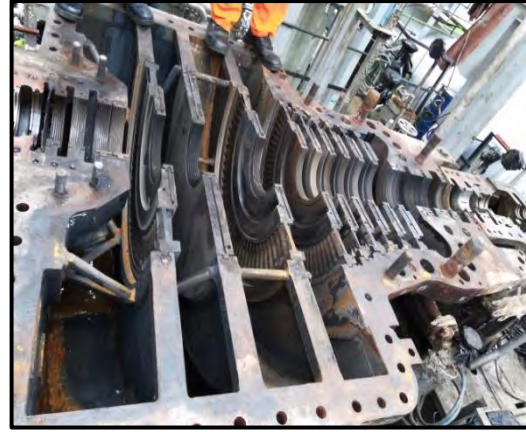
Bottom Casing Half after rotor removal
