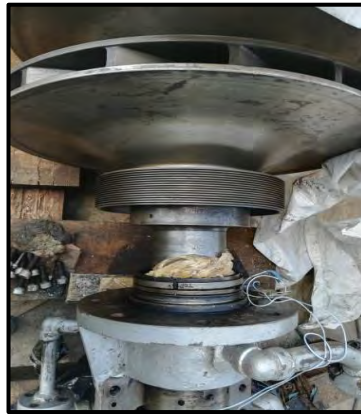
Thrust End Seal Assembly.
