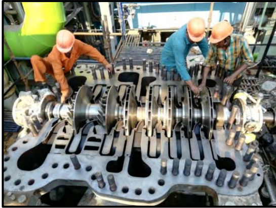
Clearance measurement & preparation for final Assy.
