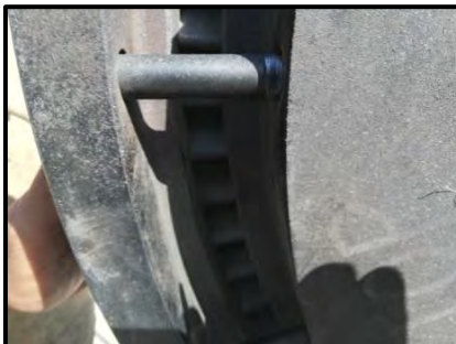
Loose diaphragm pin tack welded by SS410 welding electrode
