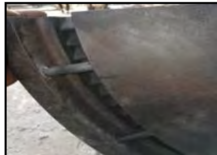
Loose diaphragm pin tack welded by SS410 welding electrode
