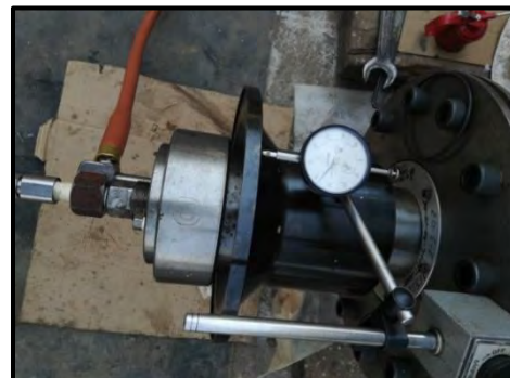
Mounting of Coupling Hub by Expander & Pusher Pressure
