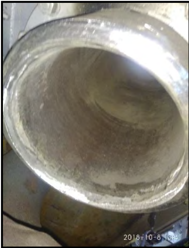
ID reduced up to 15mm of LT coil inlet header
