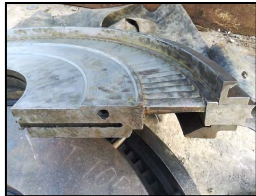
Spare 5 th stage Diaphragm with moisture ring installed
