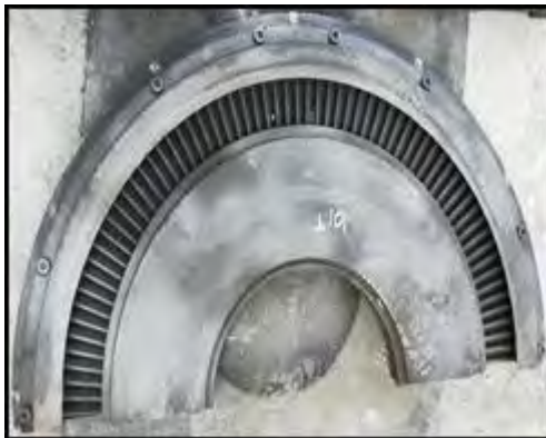
5 th stage Diaphragm with eroded moisture ring
