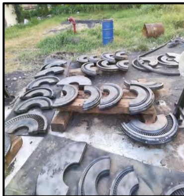
Sand Blasted Turbine Diaphragms
