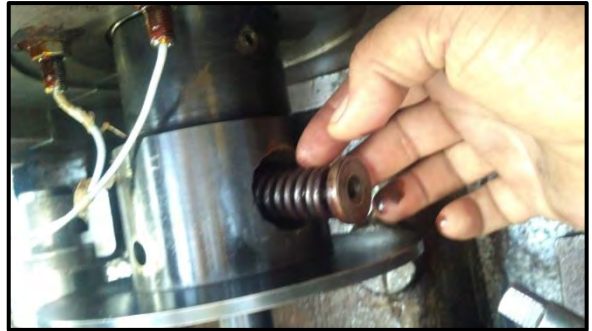
Removal of 105-JT OST assy. for cleaning & inspection
