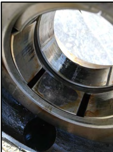
View of NDE & DE Bearing Housing after dismantling from rotor
