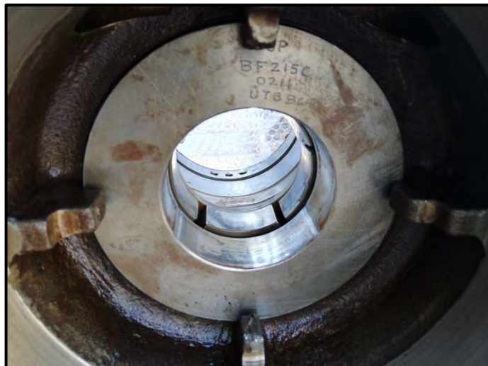
View of NDE & DE Bearing Housing after dismantling from rotor
