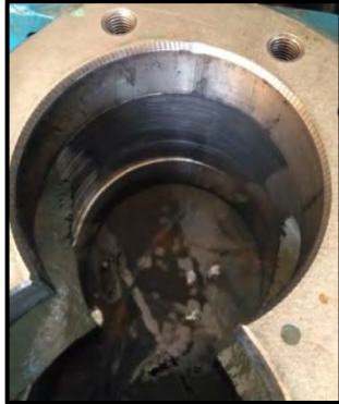
Pump Housing found worn out
