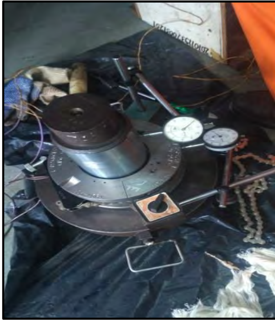
Journal Bearing Clearance measured at Mandrel
