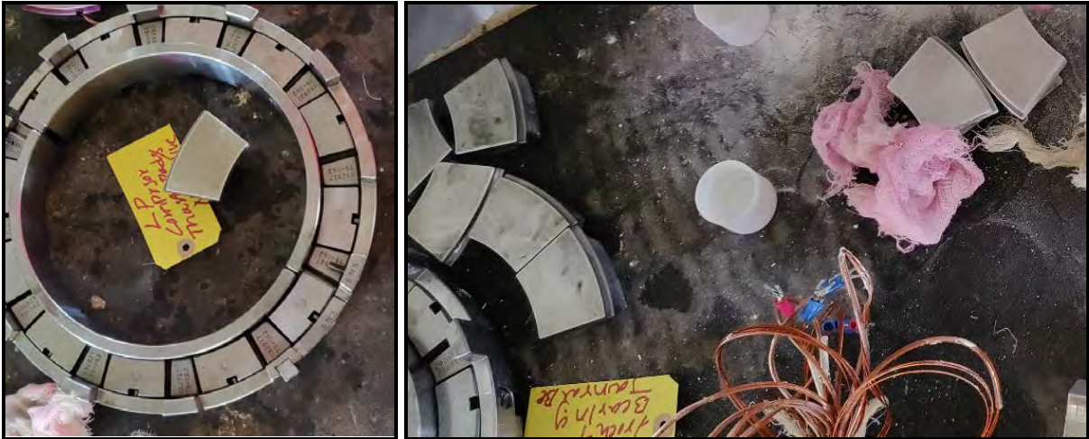
DP OF BEARINGS PADS BEING CARRIED OUT
