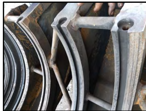
View of bottom casing half after removal of Diaphragm
