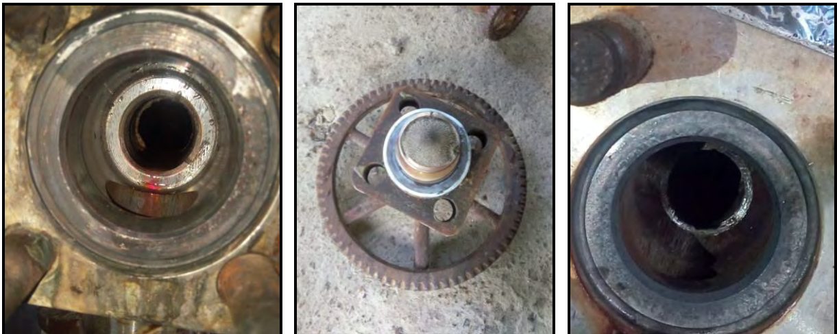
DAMAGE OF AUTOCLAVE UNLOADING VALVE SEAT & VALVE
