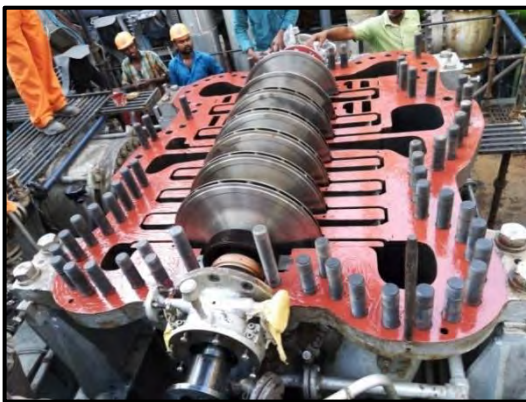
Sealing Compound applied on parting plane
