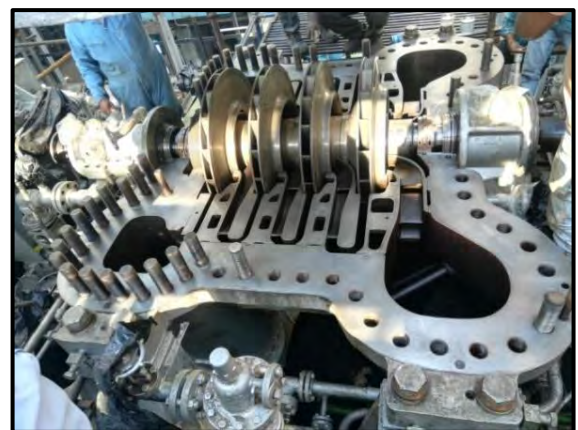
Clearance Measurement after Rotor placement & prepared for casing assembly
