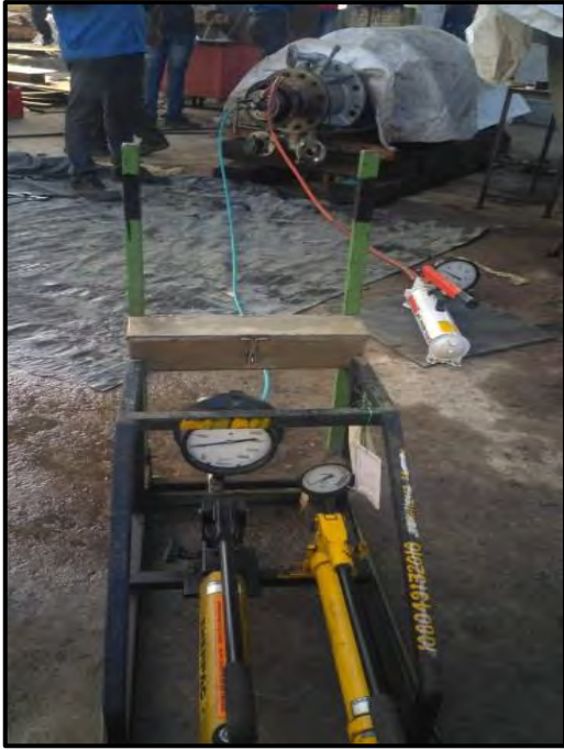
Coupling Hub Removal & Mounting Arrangement
