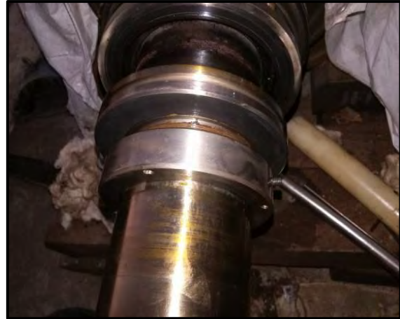
Opposite Thrust End Seal Collar Lock Nut Removal
