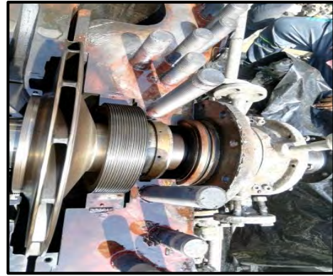
Bearing Housing and Mech. Seal Assy. at DE
