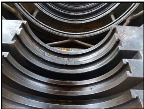
View of bottom casing half after removal of Diaphragm
