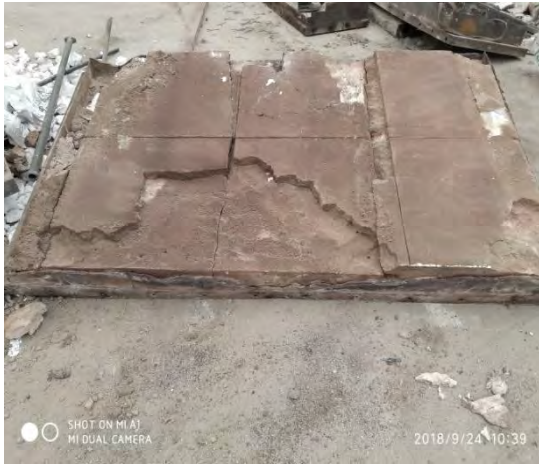
Damaged refractory of removed panel
