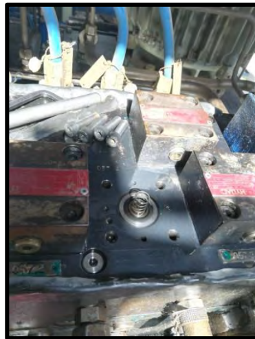
Middle Logic Cover damaged seal
