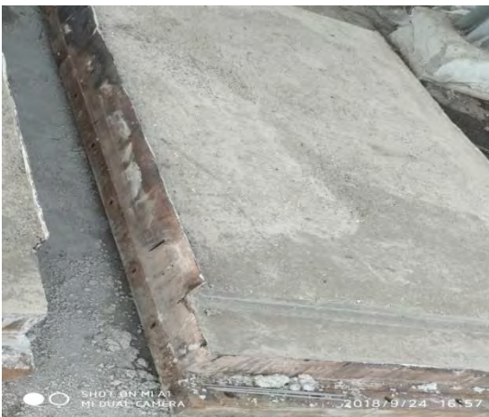
New castable Insulyte -11 in Panel
