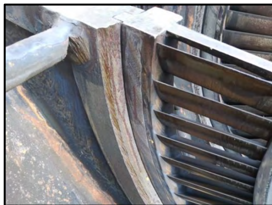
Eroded Reinforcement Rod
