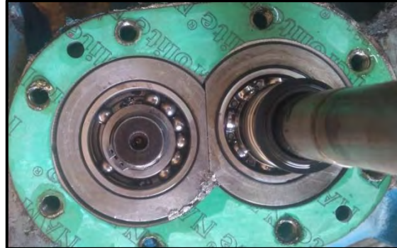
Damaged Ball Bearing
