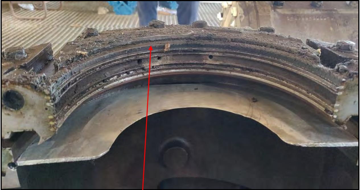
OIL COKING IN THE OUTSIDE LABYRINTH OF BEARING HOUSING OIL SEAL.
