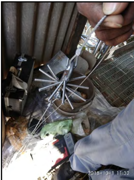
Catalyst loading by Dense loading method
