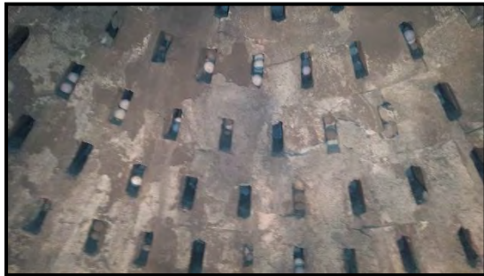
103-D bottom opening was choked by Alumina Balls
