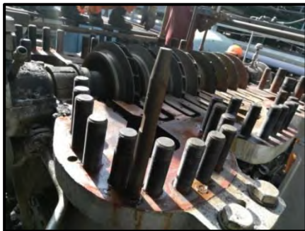
101-JHP bottom casing half after top casing half removal
