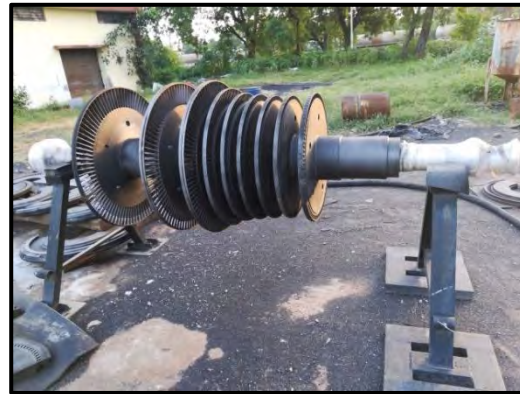
Sand Blasted Turbine Rotor
