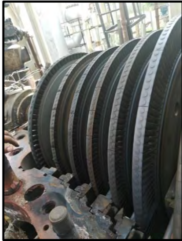
View of 101-JT after top casing removal
