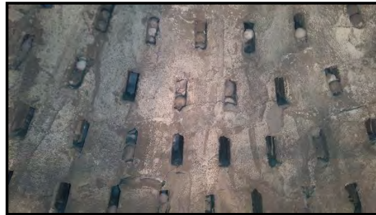
103-D bottom opening was choked by Alumina Balls
