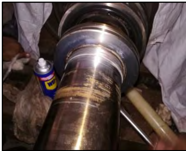
Opposite Thrust End Seal Collar Removal
