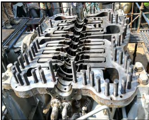
Bottom Casing Half before final assy.
