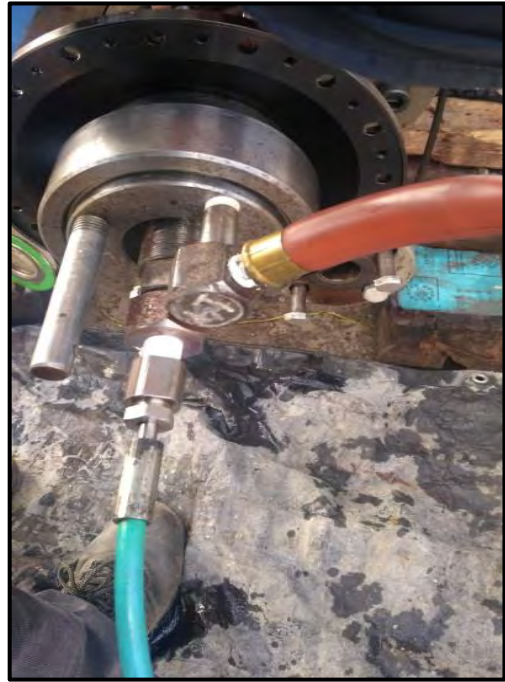
Coupling Hub Removal & Mounting Arrangement
