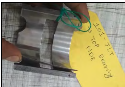
Detached White Metal Liner of NDE Bearing Top
