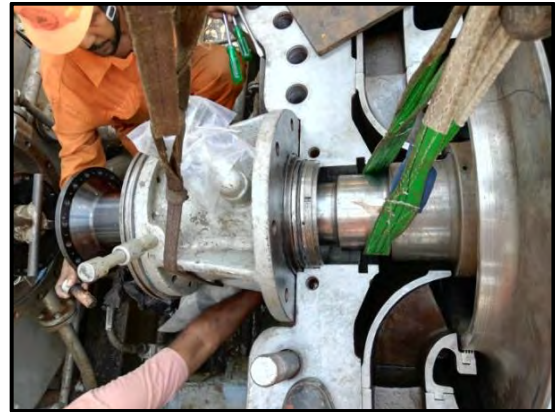
Setting of Seal at ends carefully during rotor placement
