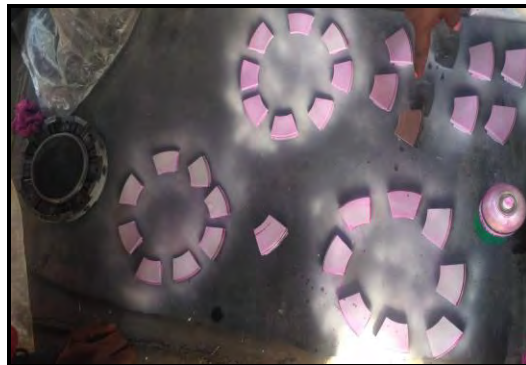
Thrust Bearing Pads DP Check
