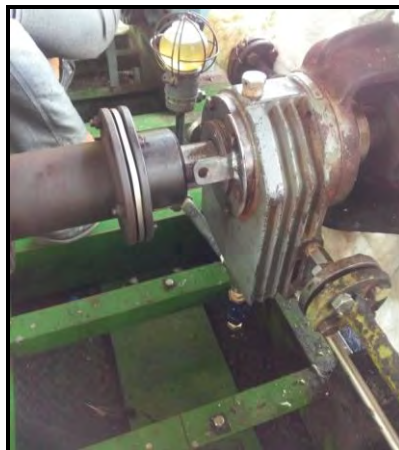
BRACKET PROVIDED ON BEARING HOUSING FOR KEYPHASOR FOR SPEED MEASUREMENT
