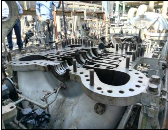
105-JLP Bottom Casing Half before Final Assy.
