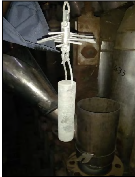
Catalyst loading by Dense loading method
