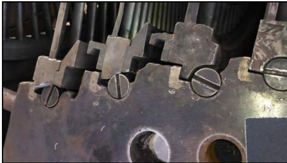
Replaced 5 th & 6 th No. Diaphragm by spare
