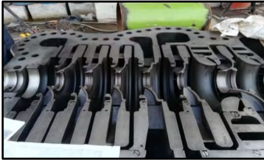
Top & Bottom Casing Half after cleaning
