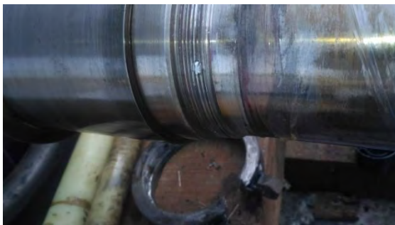
Lock Nut Set screw position
