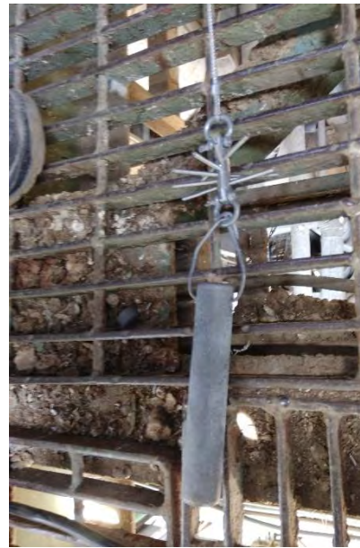
Catalyst loading by Dense loading method
