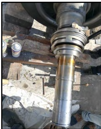
Bearing Housing Removed
