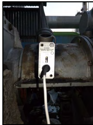
Additional Earthing brush between 101-JR & 101-JHP
