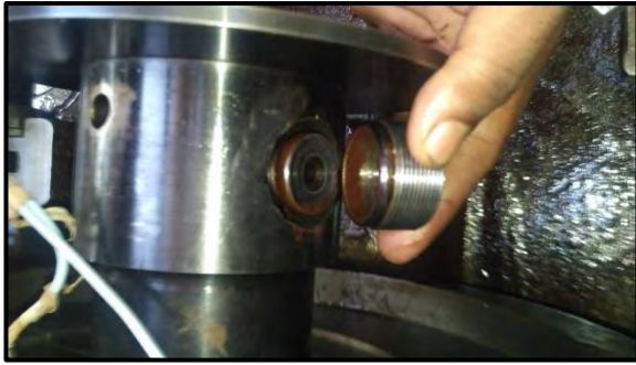
Removal of 105-JT OST assy. for cleaning & inspection
